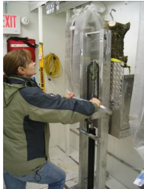
Fig. 6. Using a hydraulic lift to suspend a log from the ceiling rack.
