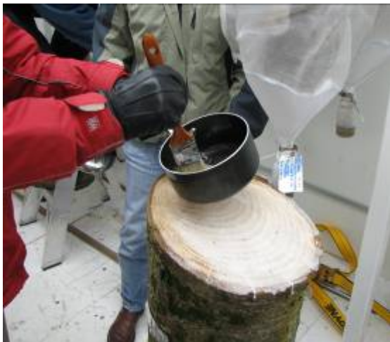
Fig. 5. Applying paraffin wax to the cut end of a log.
